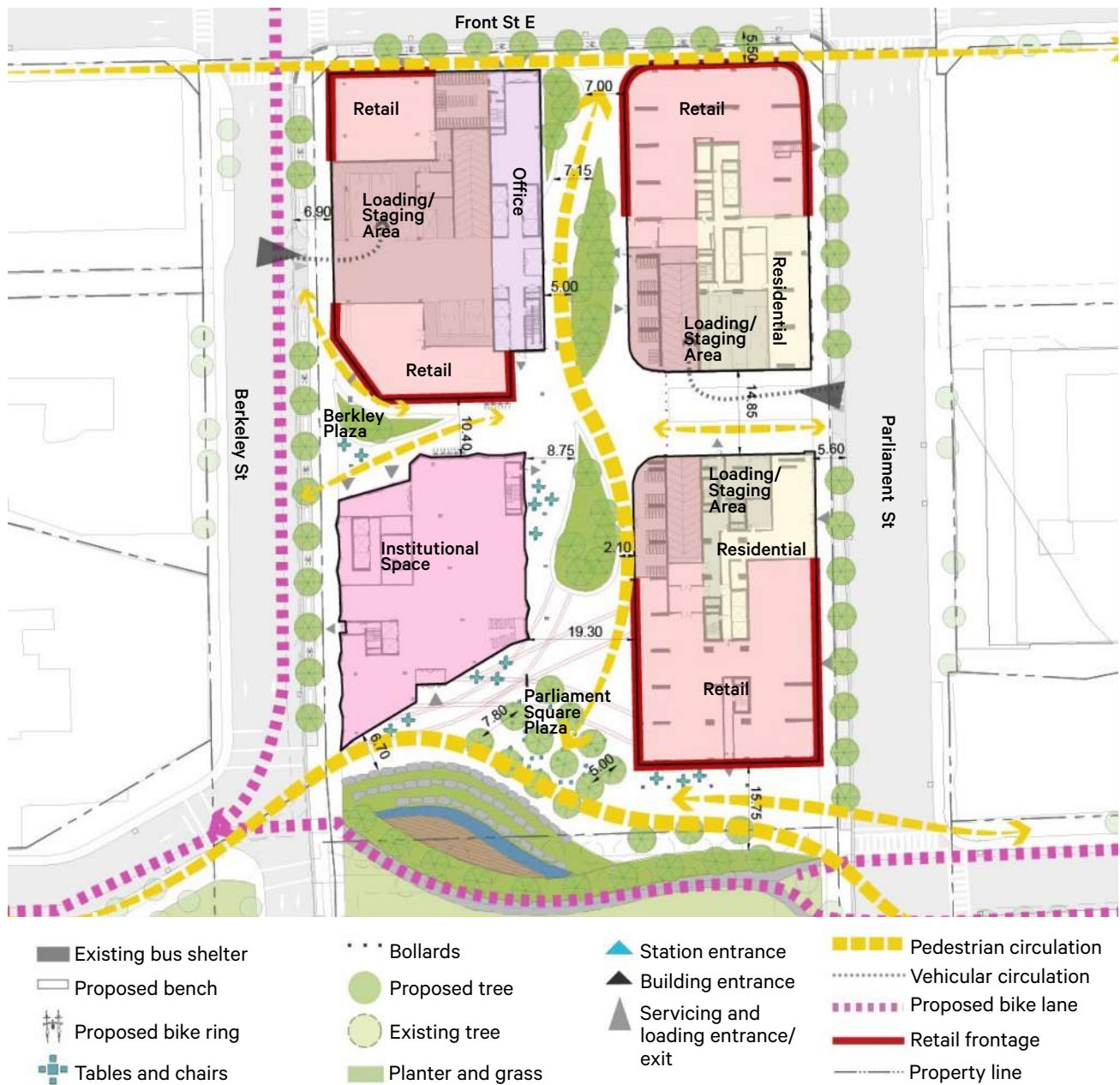
Figure 56: Front Site - Ground Level Circulation
