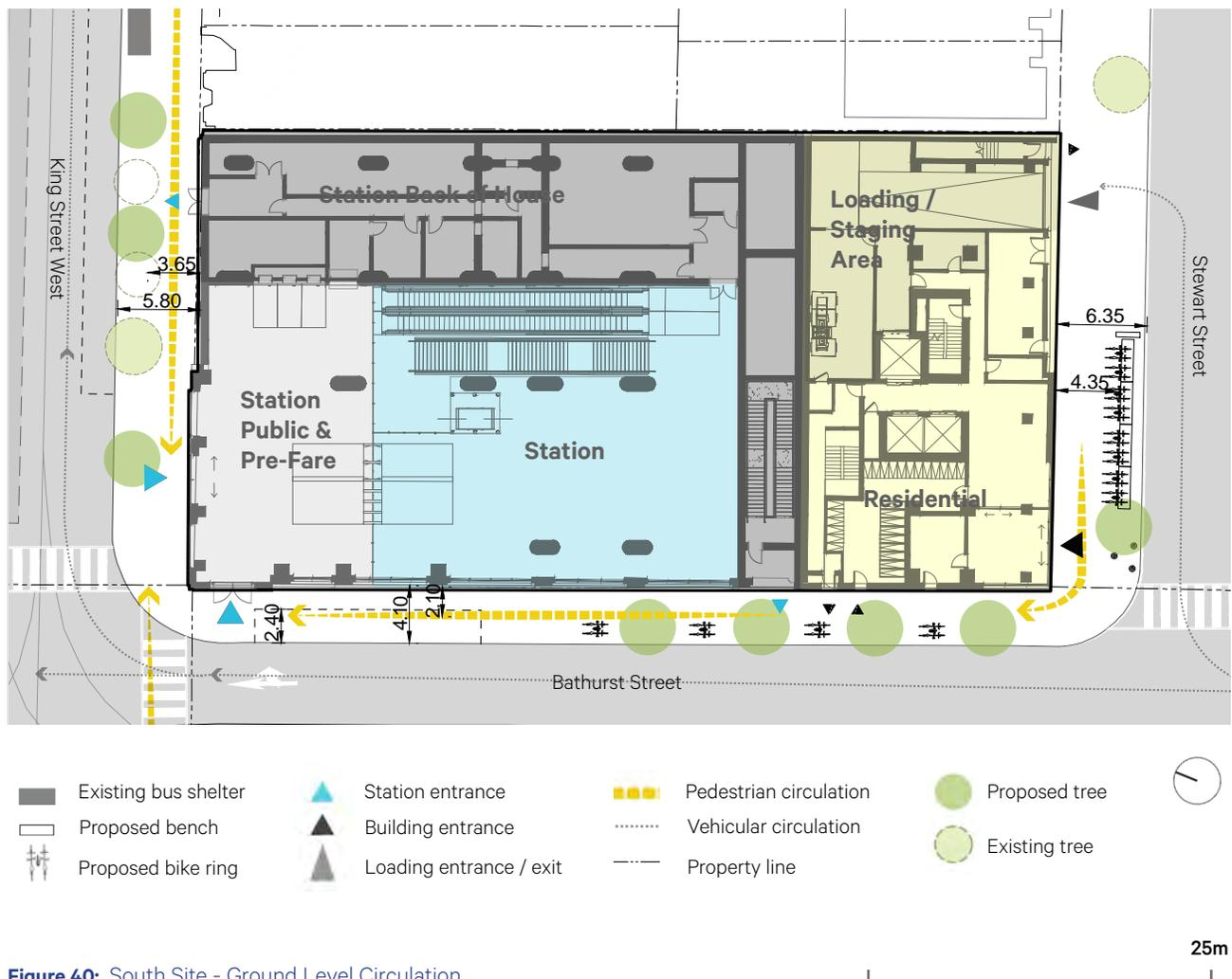
Figure 40: South Site - Ground Level Circulation
