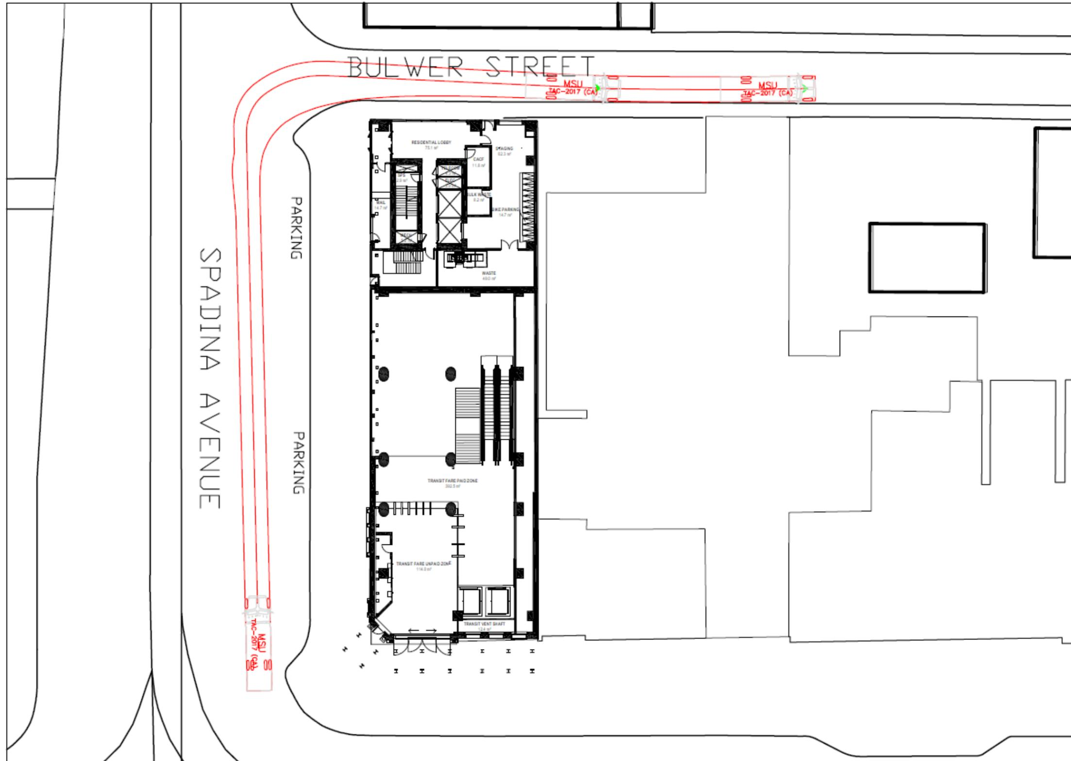
Figure 15: Loading Swept Path Analysis Medium Single Unit Truck (Northeast Corner)
