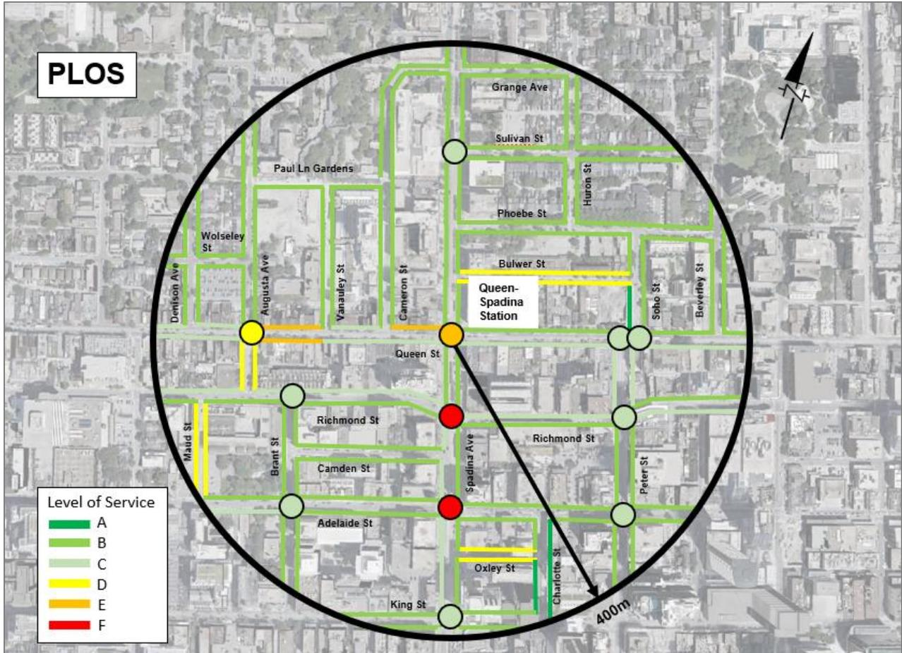
**Figure 7: Pedestrian Level of Service Analysis (PLOS)**
