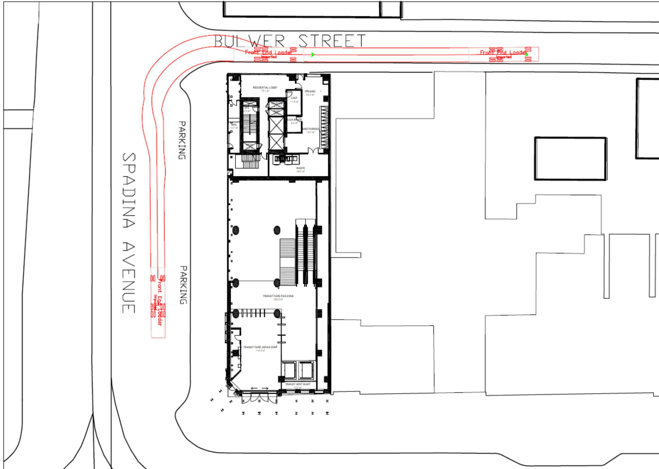
Figure 16: Refuse Swept Path Analysis Front End Loader Refuse Truck (Northeast Corner)
