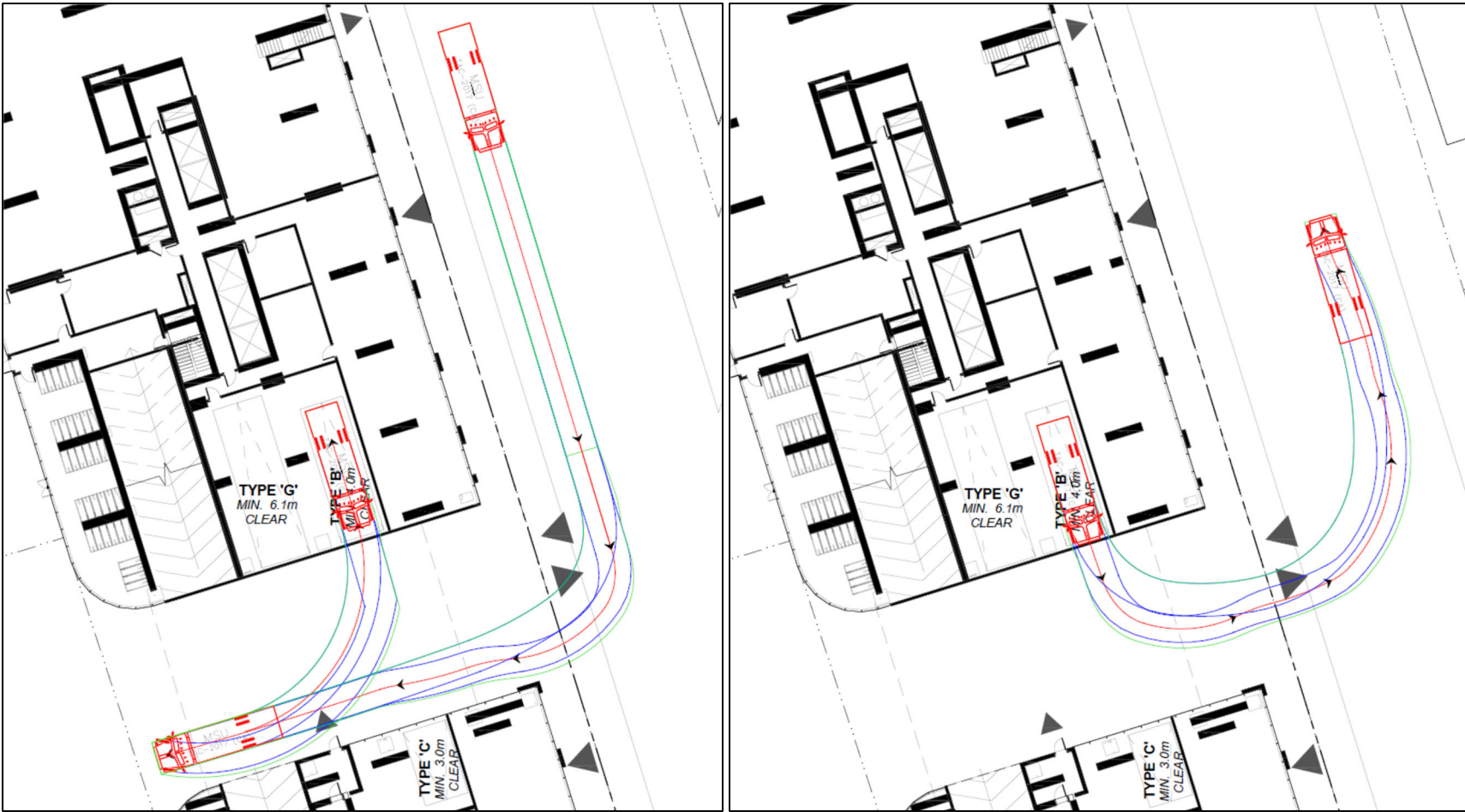
Figure 21: South Site - East Building Worst Movement (MSU)
