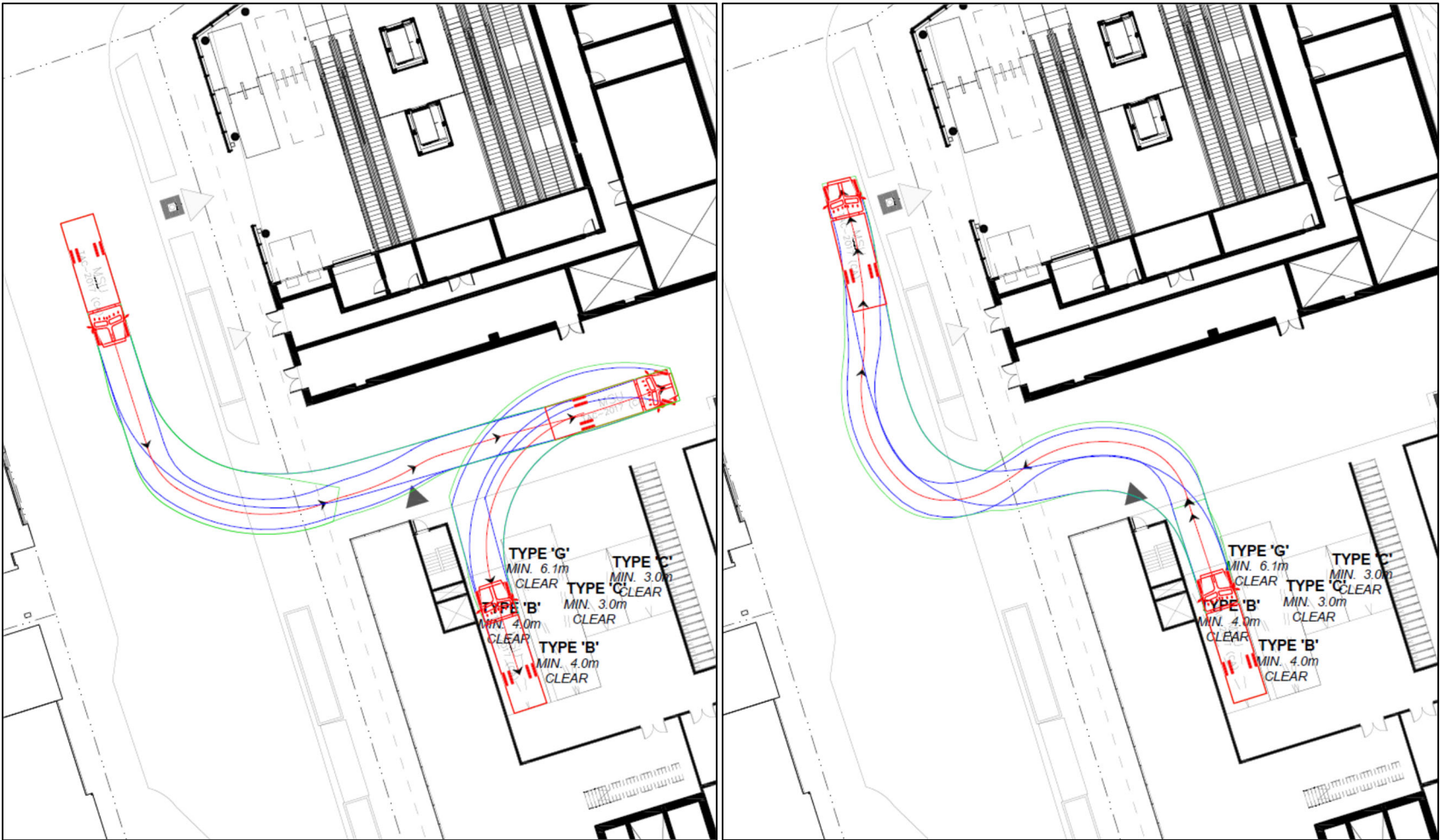
Figure 16: North Site – West Building Worst Movement (MSU)
